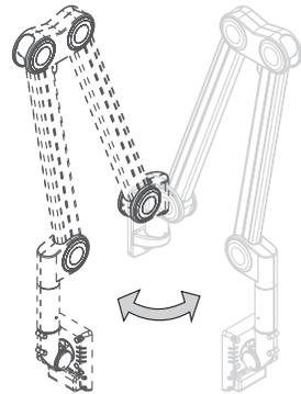
Move the arm from side to side to verify if the arm moves correctly.
