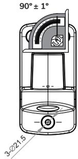
Use level gauge to help the wall mount installation.
