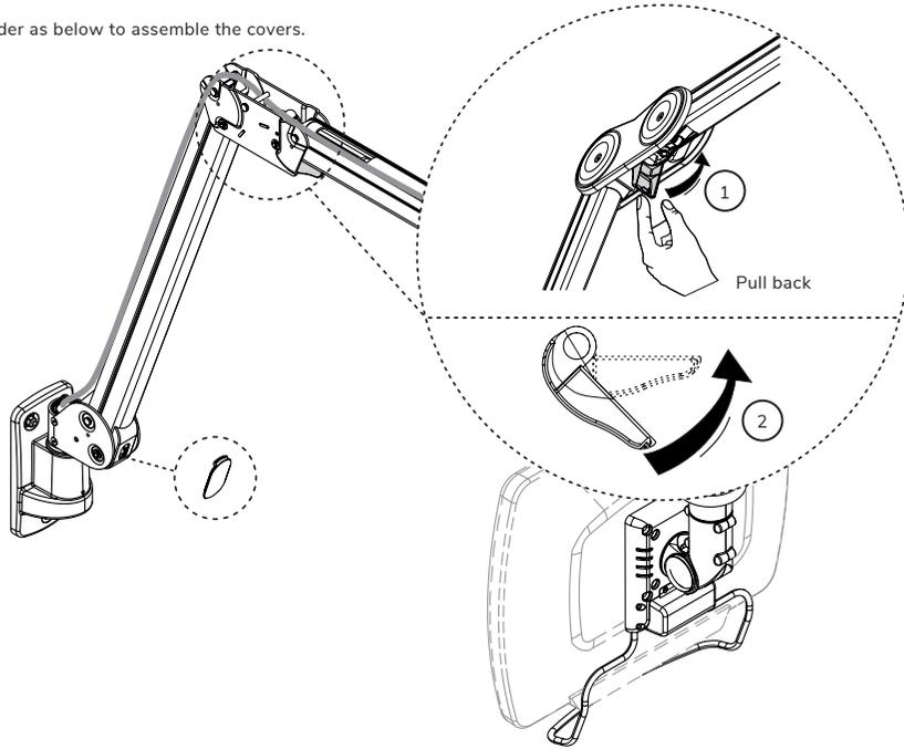
2. Carefully slide the cable covers into the slot as shown. The numbers are indicated on the inner side.
