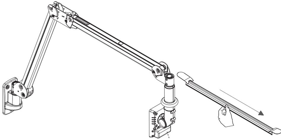
Remove the VESA cable cover with a screw driver (not provided), as shown. Keep the screws for reattachment after the monitor has been installed.
