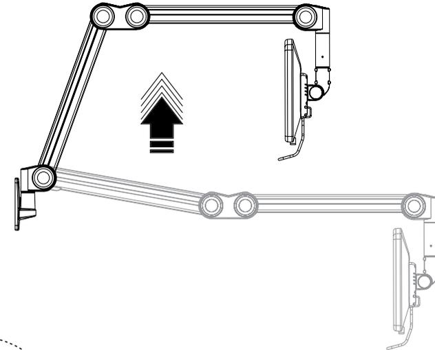
Extend the arm straight out before adjusting the weight capacity.
